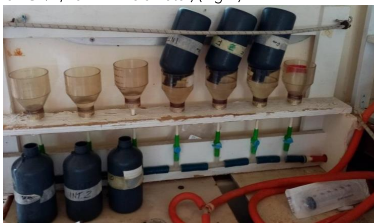
Figure 2 Filtration set up
